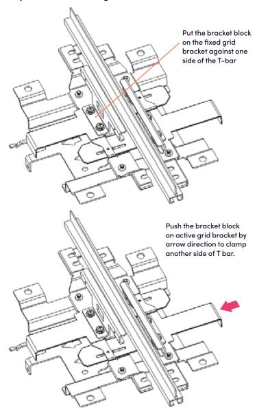
Step 4: Fix the active grid bracket and fasten two screw to prevent mounting kit from slipping
