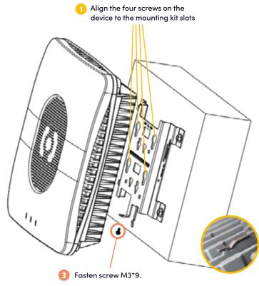
Slide the device down until the spring hook on the mounting kit meets the groove of the device
