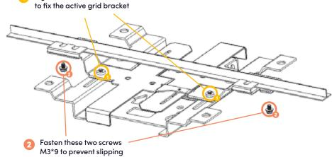
Step 4: Slide device to mounting kit, aligning the four screws and the slot.
