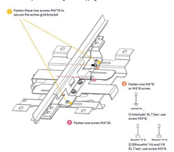
Step 5: Slide device to mounting kit, aligning the four screws and the slot.
