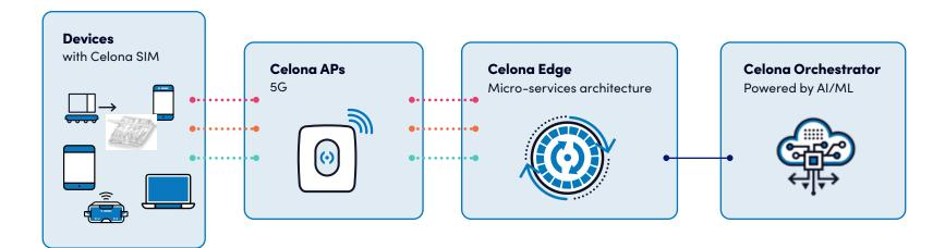
The system consists of the essential functions detailed in Figure 1: System Architecture. The Celona Orchestrator performs AP authentication, validates the AP's serial number, determines the network the AP needs to connect to and finally directs the Celona AP 22 to the serving Celona Edge.
