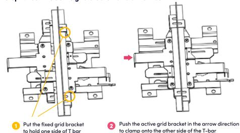
Step 3: Fix the active grid bracket and fasten the two screws to prevent the mounting kit from slipping.
