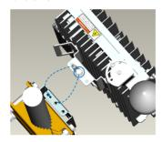
Tighten the screws on the top of the bracket on the AP using a cross screwdriver to complete the installation.
