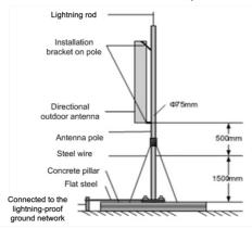
When the AP has been installed in a proper position, connect all the cables and wires. Seal and weatherproof all the connections after the testing have been successfully completed.
