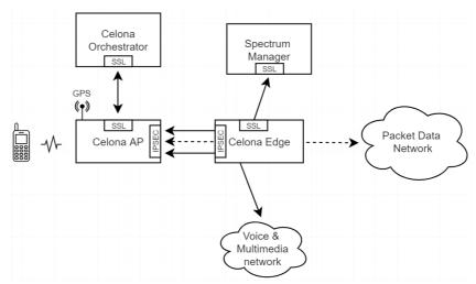
The system consists of the essential functions for a CBRS based private LTE network.
