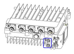
Unscrew one grounding screw, connect one end of the ground cable to the grounding screw, and fasten it again. The other end of the ground cable needs to connect to a good grounding point.
