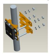
Using the 2 pins on the bracket on the back of the AP, attach the AP to the mounting bracket on the pole. Push the AP until the hook is firmly attached to the mounting bracket.
