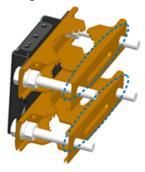
Attach the bracket to the pole, considering the height requirements above. Make sure the arrow on the installation bracket is pointing upward. Fit the threaded rod on the bracket to the pole, and then pass the two omegas through the threaded rods. Fasten with 4 flat gaskets, 4 spring gaskets, and 4 nuts.
